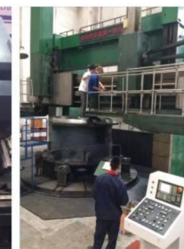
齐齐哈尔第一机床厂 五米立车改造 Qiqihar five meter vertical lathe upgraded
