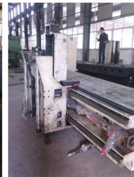
6米龙门改造 6m gantry boring and milling machine upgraded CNC Type
