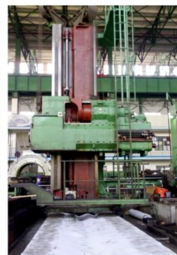
斯柯达200十米落地镗床改数控 Skoda 200 ten-meter floor boring machine changed to CNC type
