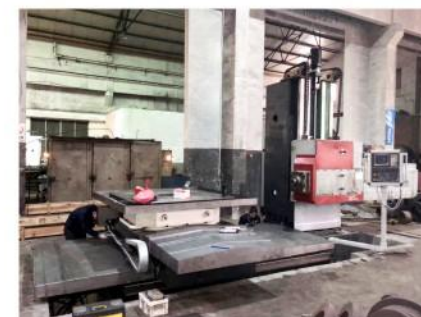
130镗床改数控 130 boring machine change to CNC type
